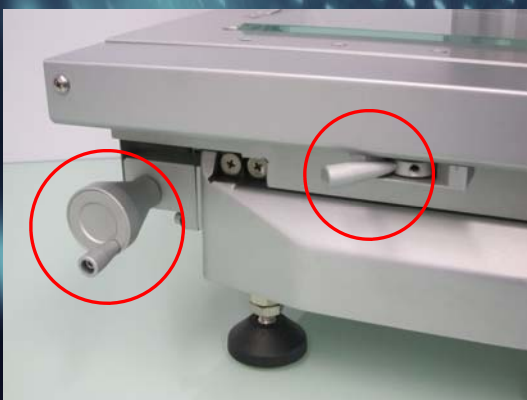
Quick release for fast stage moving in X-Y Fine movement by dial knob
