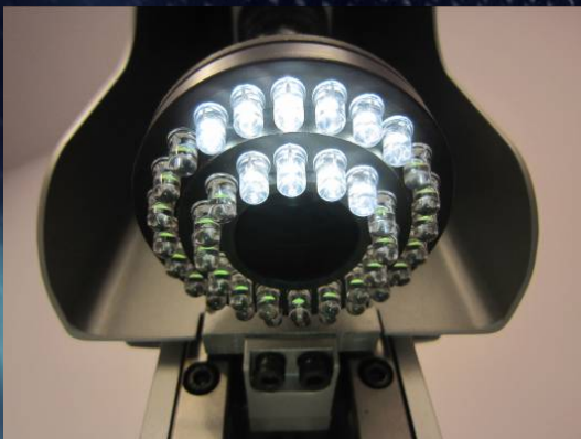
Sectional top LED ring light computer controlled for optimal illumination of your part
